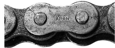
Fig. 32 Hydrogen embrittlement cracking
