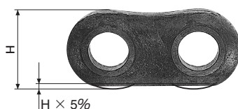
Fig. 24 Wear on the edges of the link plates
